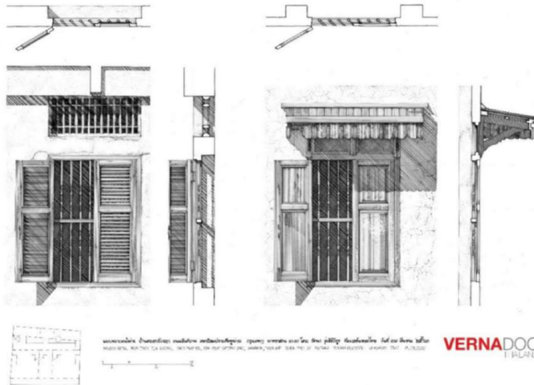
Figure 6 Baan Trok Tua Ngork: Windows detail, original scale 1/10 by Rattana Rungsiriwitoon, 2020. (VERNADOC Technique)
