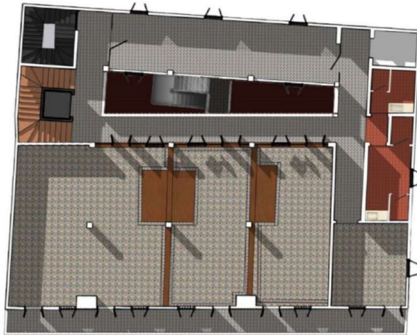
Figure 5 Baan Trok Tua Ngork: 3rd Floor Plan after the renovation by Stu/D/O Architects & Win Assakul. (Graphic: Thapakorn Boonchoo)
